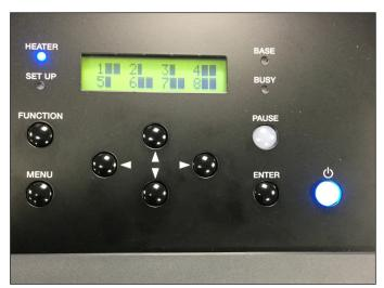
The ink indicator on the control panel displays one or two bars for the remaining ink level and lists numbers for each color instead of the actual color. It is presented in this manner because ink colors can be positioned in different slots on the device, depending on its ink color configuration.
