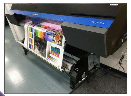
The take-up system, which is optional with the TrueVIS VG-640, enables multiple jobs to be readily collected onto a core facilitating unattended print runs.
