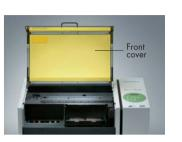
used in conjunction with delicate materials which, traditionally, have been difficult to dry efficiently. The LEF-12i includes a safety hood to protect the operator from UV light during operation and a screen to prevent dust falling on the surface of materials whilst printing.
